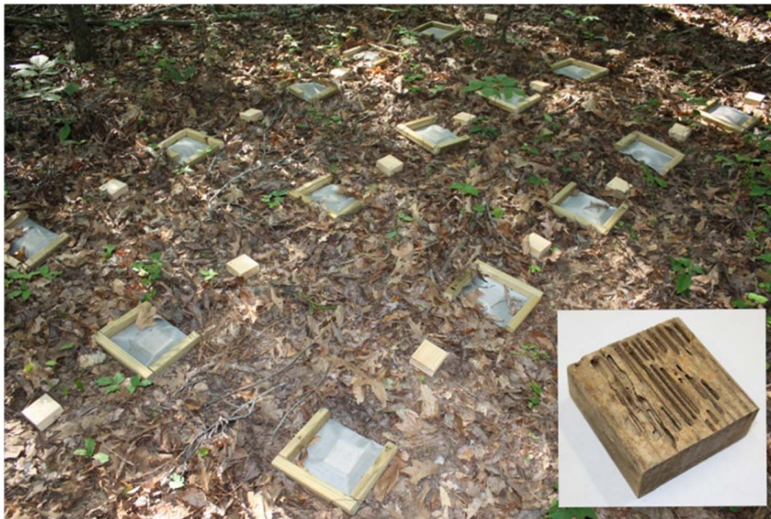
Figure 3. Protected and unprotected blocks without termite damage were used to determine how the mesh bags affected water content beyond the exclusion of insects. An unprotected block with Reticulitermes damage is shown in the inset. doi:10.1371/journal.pone.0101867.g003
