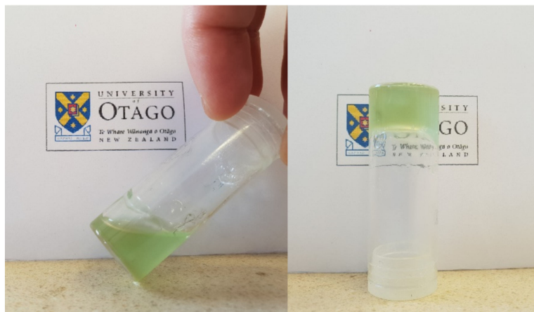
Figure 3. Gelation of a 30% solution of PEO 8 -40k-PDEGA (P5) on warming to RT from 0 °C.
