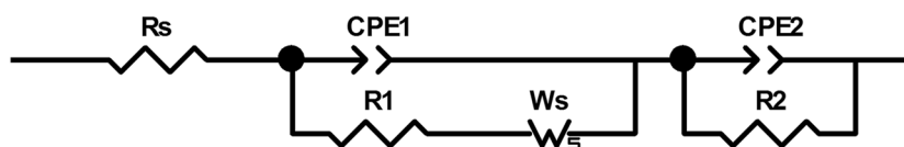
Figure 7. Equivalent electrical circuit used for fitting the EIS experimental data.
