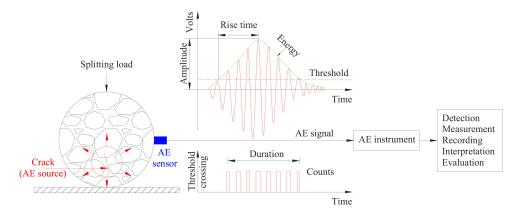
Figure 3. Schematic diagram of AE monitoring under indirect tensile load.
