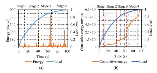
Figure 8. The energy and cumulative energy distribution of OGFC: (a) energy; (b) cumulative energy.
