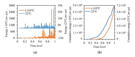
**Figure 10.** The energy and cumulative energy distribution of AC at -10 °C and 25 °C: (**a**) energy; (**b**) cumulative energy.
