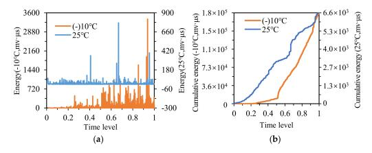
**Figure 12.** The energy and cumulative energy distribution of OGFC at -10 °C and 25 °C: (**a**) energy; (**b**) cumulative energy.
