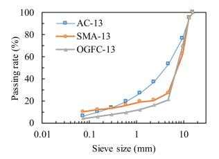
Figure 1. Selected gradation of AC, SMA, and OGFC.
