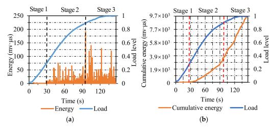
Figure 6. The energy and cumulative energy distribution of SMA: (a) energy; (b) cumulative energy.
