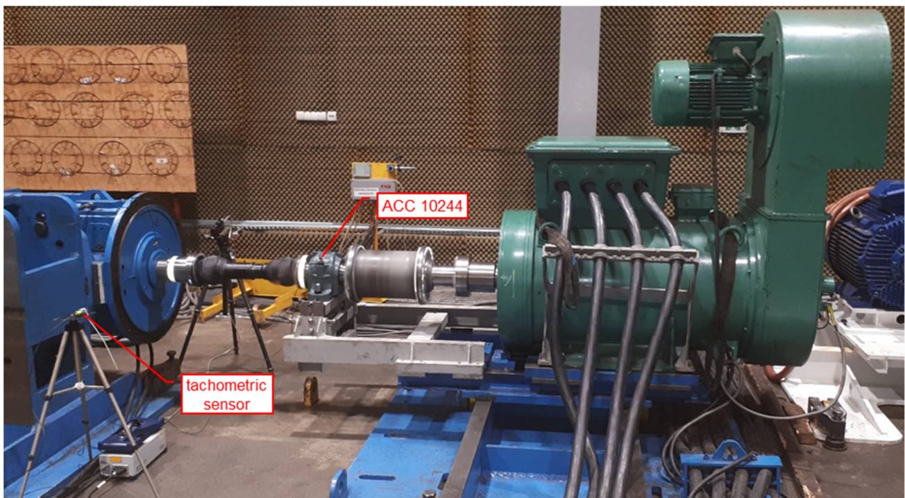
Figure 8. Location of the vibration and tachometric sensors used for the analytical experiment.
