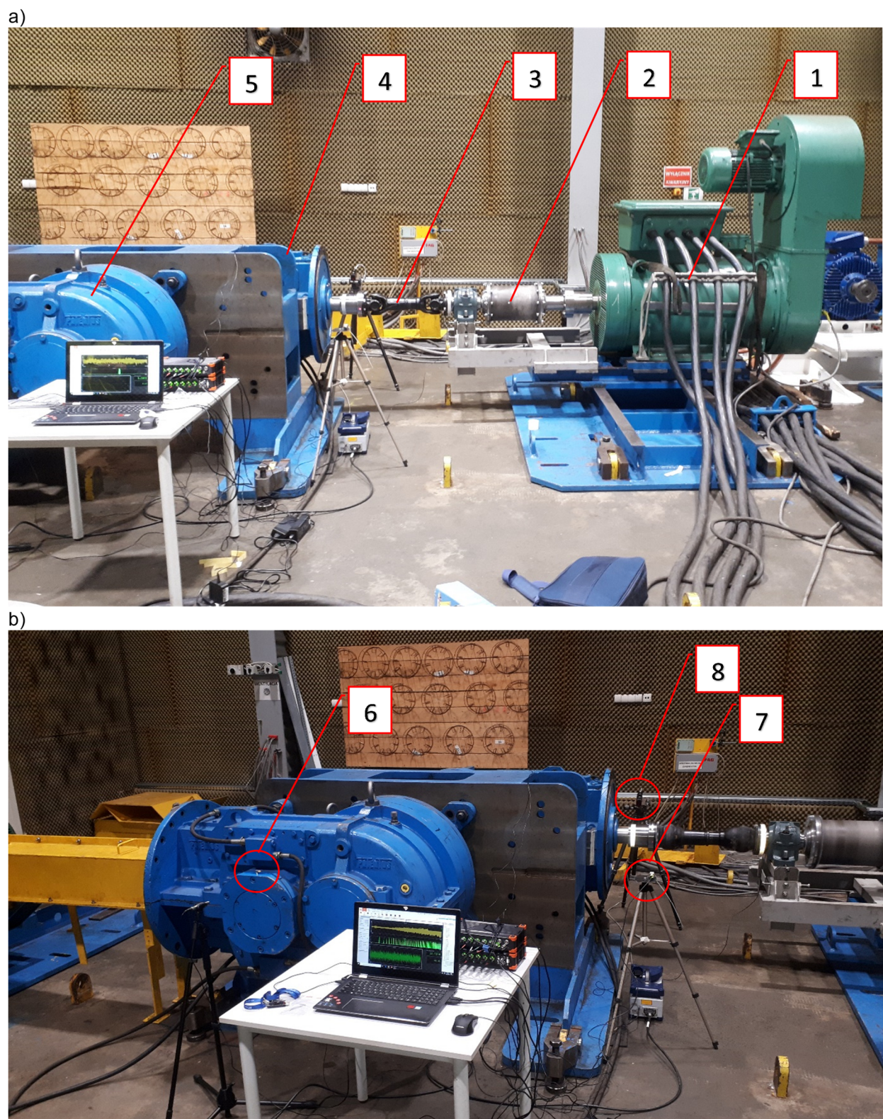
Figure 1. Object of the research: electric motor driving (1), innovative flexible torsion clutch (2), shaft with universal joints (3), set of two multistage gears ((4) and (5)), vibration acceleration converter (6), tachometric sensor (7), and laser vibrometer for non-contact laser measurement of instantaneous angular velocity changes of the shaft by Polytec RLV-5500 (8)—(a,b) represents different view.
