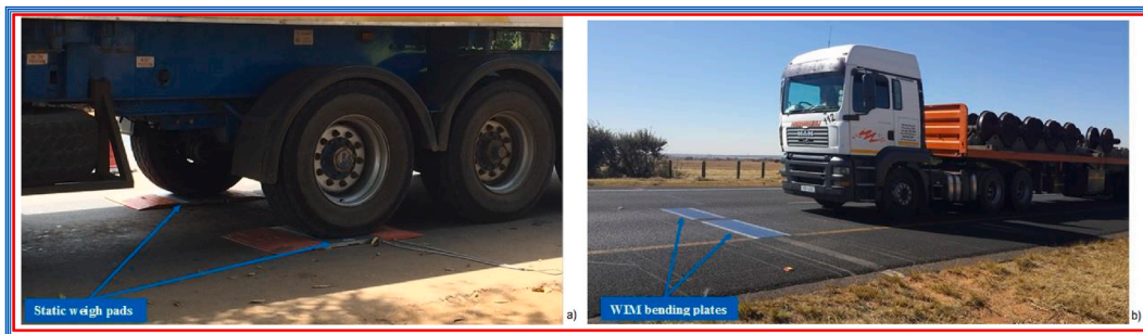
Fig. 5. Weighing materials. a) Portable static weigh pads; b) Weigh-in-motion bending plates [10].
