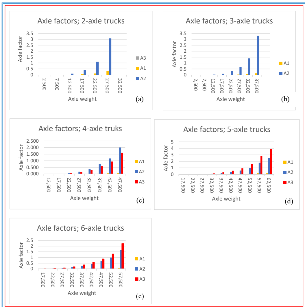
Fig. 13. AF distribution for different trucks. a) 2-axle trucks; b) 3-axle trucks; c) 4-axle trucks trailers; d) 5-axle trucks; e) 6-axle trucks.
