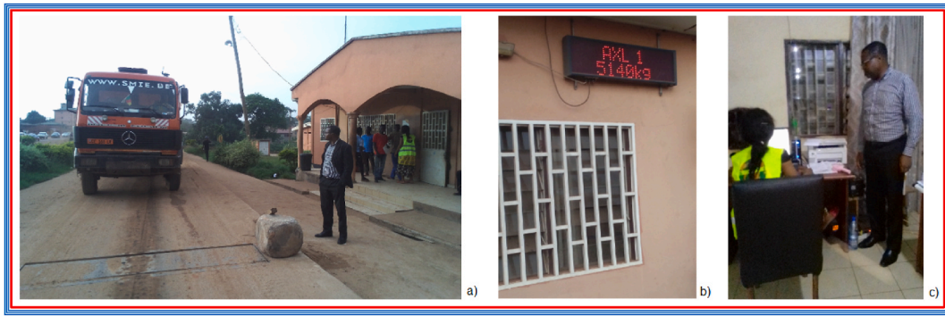
Fig. 6. Mezos Fixed static weigh (FSW) on national road n°1 Yaounde – Obala. a) Weigh pad; b) displayed board; c) working station.
