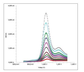
Fig. 7: Square wave voltammograms for different concentrations of etodolac.
