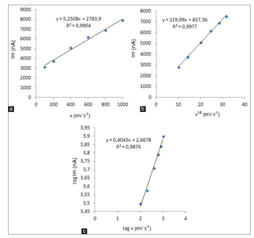
Fig. 4: Dependence of peak current on the scan rate (30  $\mu$ g/ml). a and b are different scan rates and c is logarithmic scan rate.
