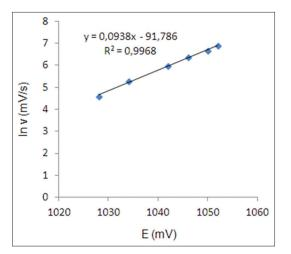
Fig. 5: Dependence of anodic peak potentials of voltammetric peak for the oxidation of  $30 \mu g/ml$  etodolac on the scan rate.
