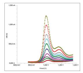
Fig. 8: Differential pulse voltammograms for different concentrations of etodolac.
