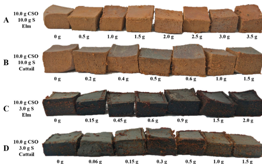
Figure 3. Picture of bio-based polysulfide composites prepared with different fillers. (A) 10.0 g CSO + 10.0 g S + elm, (B) 10.0 g CSO + 10.0 g S + cattail, (C) 10.0 g CSO + 3.0 g S + elm, (D) 10.0 g CSO + 3.0 g S + cattail.
