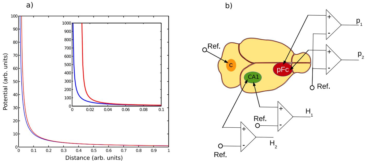
**Fig 3.** a) Example of potential measured in  $P_1$  and  $P_2$  versus distance  $r$  in normalized units. One notes the strong similitude between  $P_1$  and  $P_2$  when  $r$  is large in comparison with the distance shift  $\varepsilon$  of the two electrodes. Also, we observe a strong amplitude difference between potential  $P_1$  and  $P_2$  when the current source is close to the electrodes pair (zoom in figure). b) Recording methods and electrodes location during the experiment.
