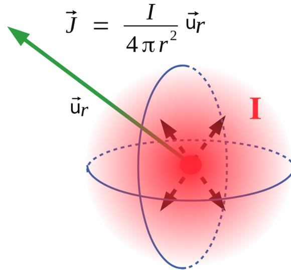
**Fig 1. Current source:** A current in an homogenous medium yields a current source density flowing in all directions. The current density writes:  $\vec{J} = \frac{I \vec{u}_r}{4 \pi r^2}$ , where  $r$  is the distance to the current source and  $I$  the current generated at the origin. The Ohm law ( $\vec{J} = \sigma \vec{E}$ ) leads to the potential  $V = \frac{I}{4 \pi \sigma r}$  created at any distance  $r$ .
