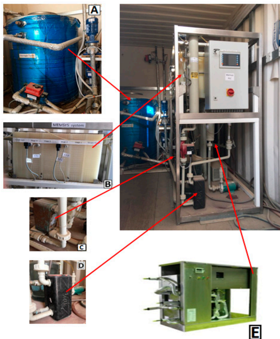
Figure 1. Photographs of the V-MEMD system facilities. (A) Thermal storage tank, (B) multiple effects, (C) HX-2, (D) HX-1, and (E) heat pump system.
