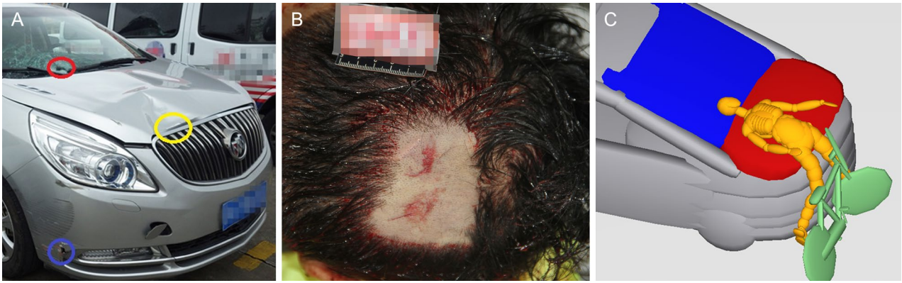
Figure 1. (A) Damage on the vehicle involved in the collision, (B) occipital region scalp lacerations on the cyclist, and (C) the instant of head–windshield impact in the result that showed the most likely scenario. Adapted with permission from [82].
