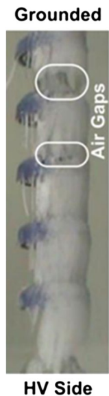
Figure 2. Surface performance of iced insulator strings.
