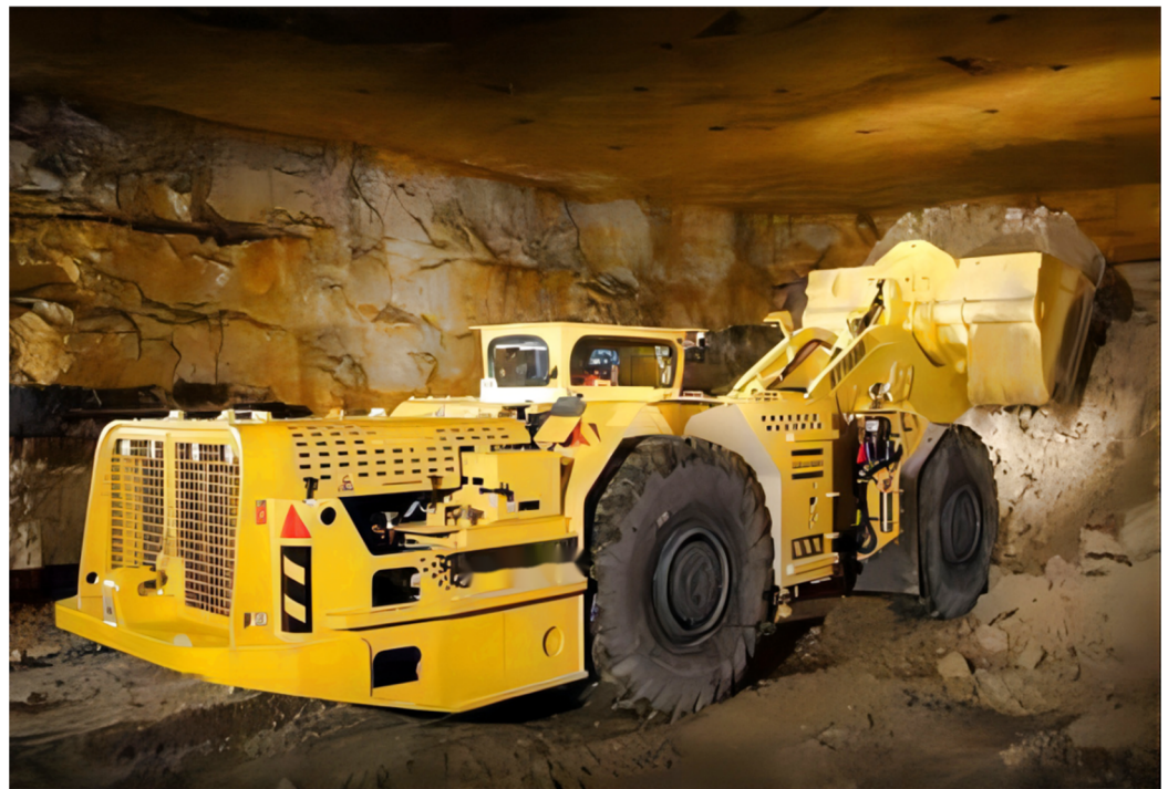
Figure 1. Track-less transport vehicle: the underground scraper (LHD).
