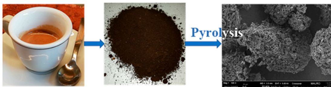
Figure 1. Conversion process of brewed coffee waste to carbon material.
