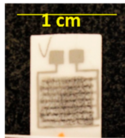
Figure 2. A picture of a CGB sensor screen printed sensor.
