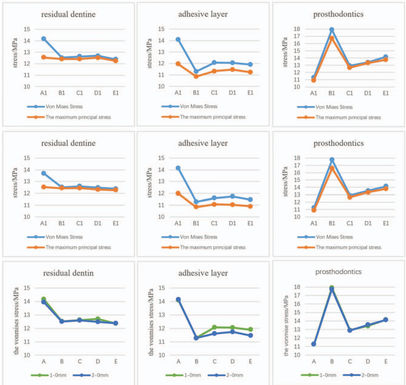
Figure 3. The Von mises stress value and the maximum principal stress value of each layer in each model.
