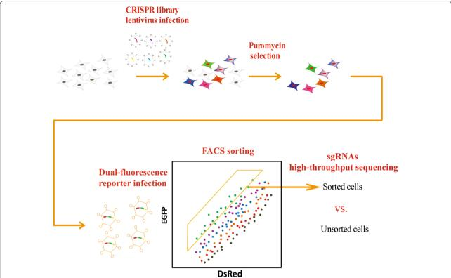
**Fig. 1** The workflow of the protein stability regulators screening assay (Pro-SRSA). *CRISPR* clustered regularly interspaced short palindromic repeat, *FACS* fluorescence-activated cell sorting, *EGFP* enhanced green fluorescence protein, *DsRed Discosoma* sp. red fluorescent protein, *sgRNA* single-quide RNA
