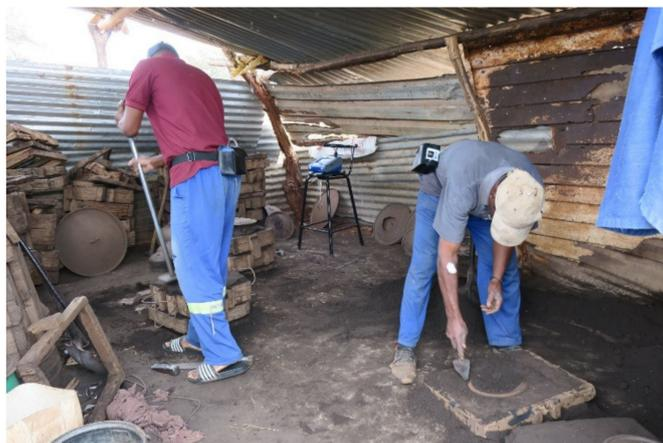
**Figure 1.** One of the hand-made cookware operation sites with artisans preparing sand mold.
