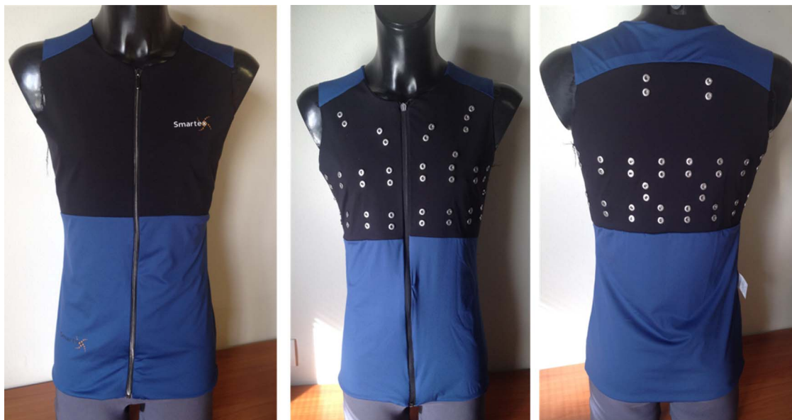
Figure 3 The proposed concept vest and sensors for Wearable Sensing and Smart Cloud Computing for Integrated Care to Chronic Obstructive Pulmonary Disease Patients with Co-morbidities (WELCOME) system. Acknowledgement Smartex s.r.l.
