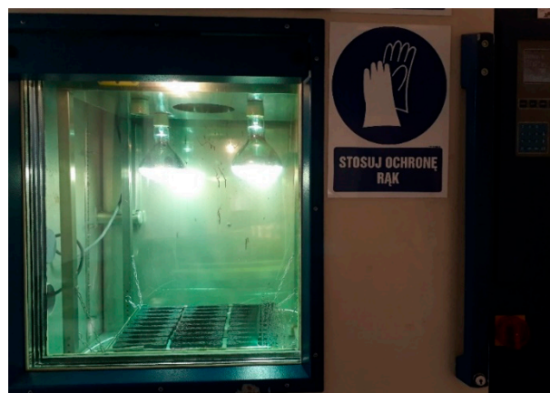
Figure 10. Samples of the elastomeric material in the climatic chamber Feutron, simulating high temperature and solar radiation.
