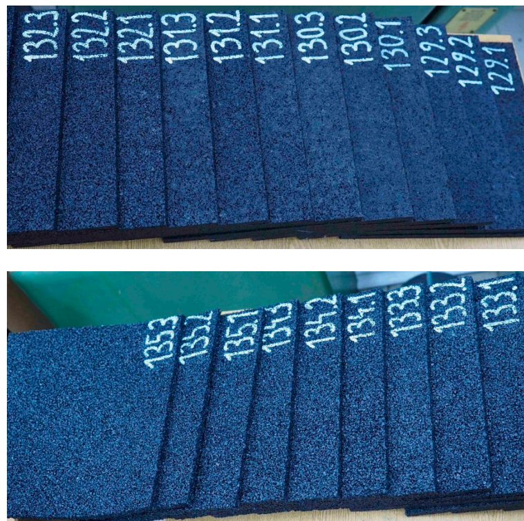
Figure 2. SBR samples with visible porosity increase for the materials with lower densities (higher numbers).
