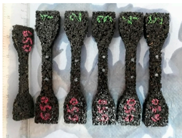
Figure 17. Change of length for sample SBR 650 after 7 days in oil.
