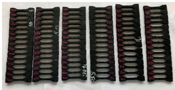
Figure 9. Samples of the elastomeric material with various densities prepared for ageing tests (high temperature and UV radiation).
