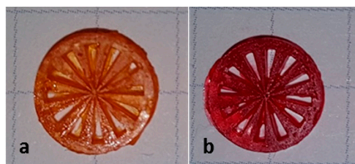
Figure 19. Green bodies of Siemens stars produced by LCM, using Disperse Orange 3 (a) and Sudan IV (b).
