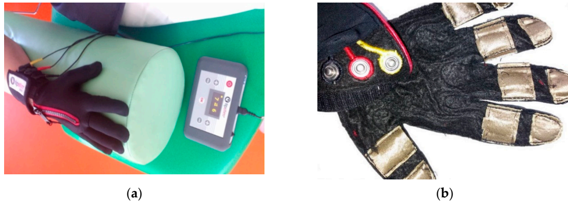
Figure 5. Electrostimulation therapy kit using the TipStim glove: (a) medical stand; (b) the internal view of stimulation glove.
