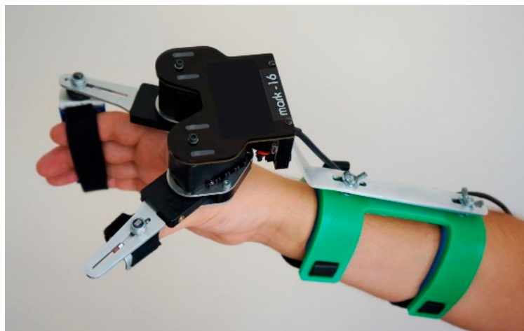
Figure 2. Example of a rehabilitation hand robot constructed in Poznan University of Technology.
