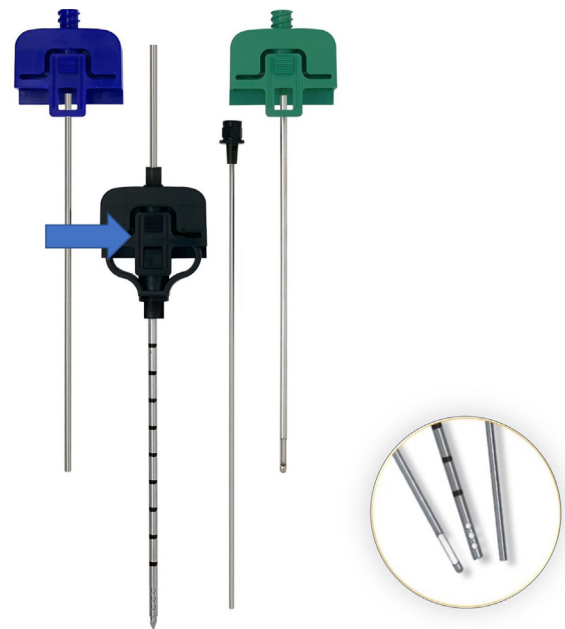
Fig 2. The Tactoset® system contains an 11-gauge, black-handled, drillable outer pin. The blue arrow indicates the cannula lock, which always faces the direction of the side-delivery holes at the end of the cannula. Once in the appropriate location, the inner sleeve of the pin can be removed to allow for either a single end delivery (blue) or 3-hole side delivery (green) of the injectable. A metal push rod is available to remove the excess calcium phosphate from the chamber of the delivery pin.
