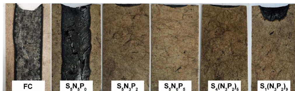
Figure 3. The residual carbon layer sample after a horizontal combustion test.
