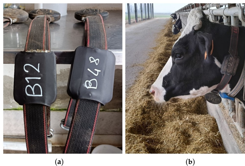
Figure 4. (a,b). Two sensor nodes mounted on two neck-collars (with the identification code written by pen) (a) and the position of the collar on the neck of a cow (b).
