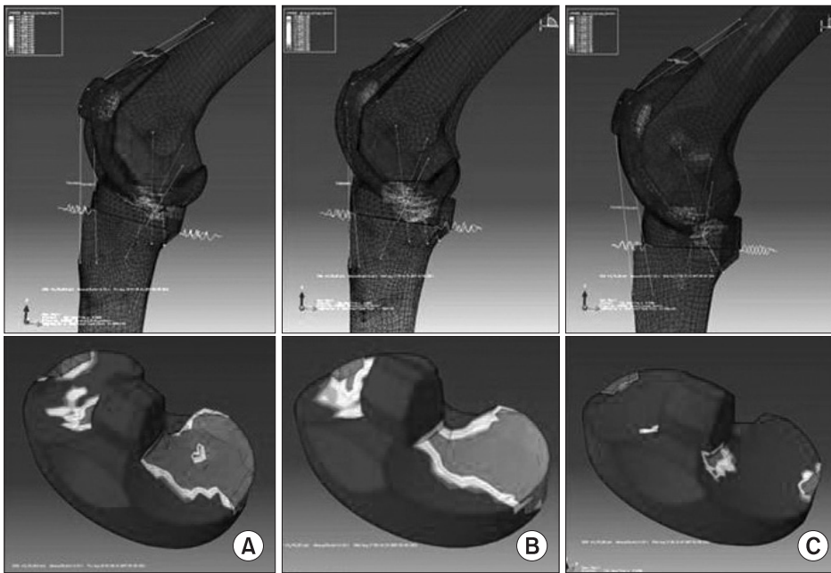
Fig. 6. Stress distribution on bearing for total knee replacement with posterior tibial slope of (A) 10° (B) 7° (C) 0° under 60% gait cycle.
