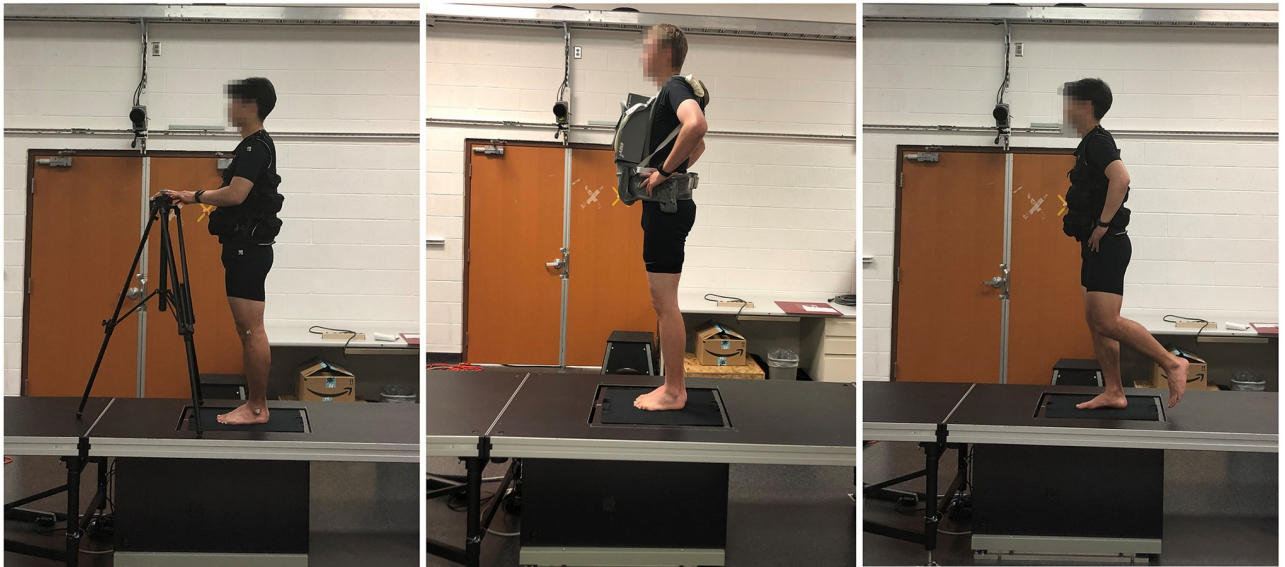
Fig 1. Raised platform/walkway, weight conditions, and standing tests. Left: Static trial with evenly distributed (EV) weight. Middle: Bilateral-foot standing trial with front weight (FV). Right: Single-foot standing trial with EV.
