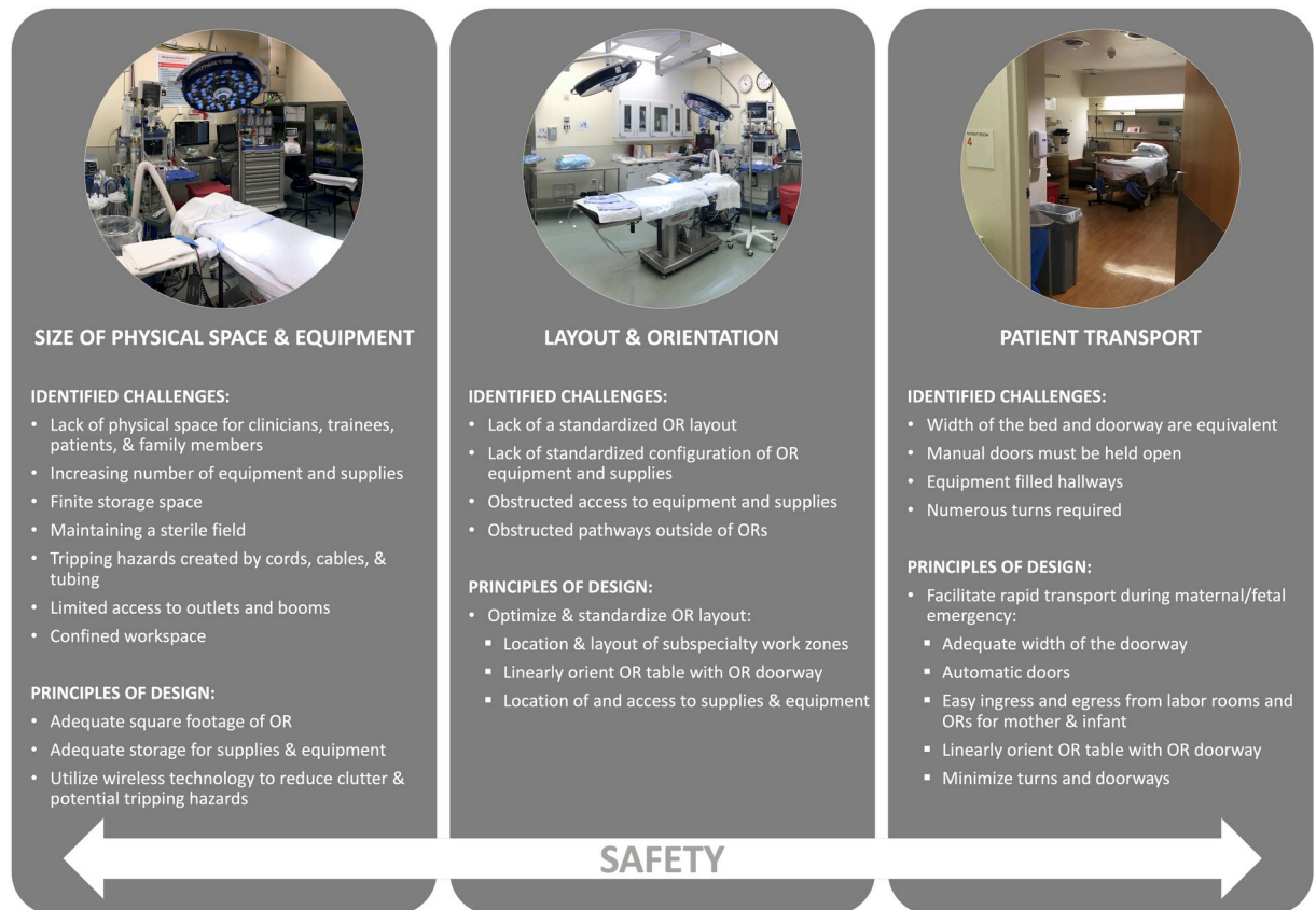
Fig 5. Key points: Identified challenges during an emergency Cesarean and relative principles of design.
