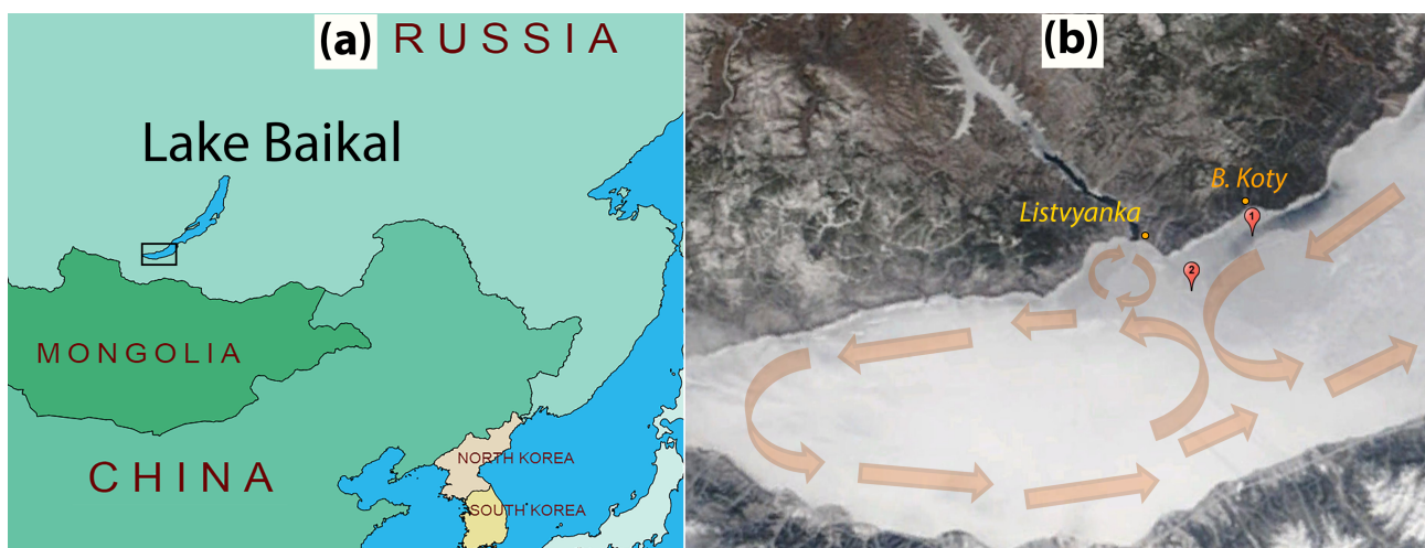
Figure 7. (a) Geographical location of the study site; (b) Ice conditions at the end of the experiment (on 31 March 2014) with the pattern of mean currents according to [34] in the southern part of Lake Baikal and locations of the autonomous measurement stations. The satellite image (Terra MODIS true color band composition) obtained from the Irkutsk Center of Remote Sensing [35]. Note the stronger ice melt in the area of the jet current around Station 1 visible as a dark area in Panel (b).
