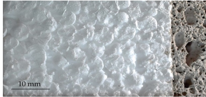
Figure 8. Section of the polystyrene board with a layer of S20. Three experimental tests were conducted with specimens 20, 15, and 10 mm thick.
