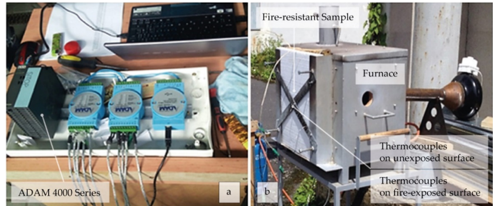
Figure 3. Equipment setup for monitoring the temperature variations: (a) ADAM 4000 Series and (b) internal (K5–K9) and external thermocouples (K1–K8).
