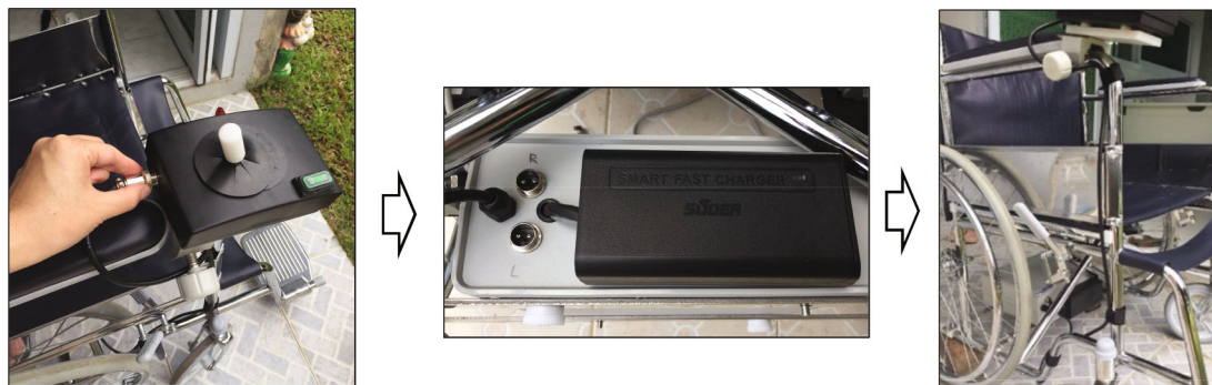
FIGURE 9: Connecting all of the main parts with a set of electric wire.
