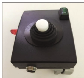
FIGURE 5: The direction controller of the prototype for the simplified power wheelchair.
