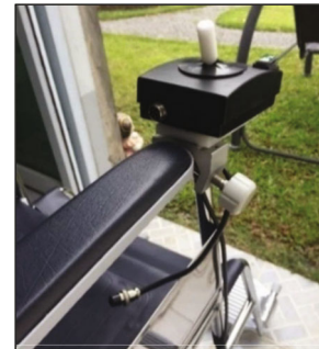
FIGURE 8: Setting up the direction controller.
