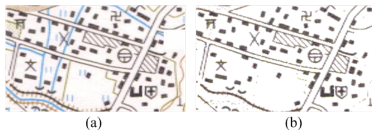
Figure 2. The figure shows the comparison of map changes after color segmentation, as follows: (a) the original image of the topography map; (b) the sub-layout images of the topography map.
