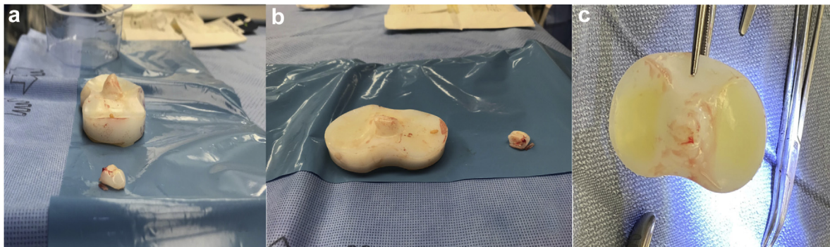
Figure 3. Intraoperative images from a revision BCS TKA displaying a 14-mm Journey 1 BCS explanted tibia polyethylene with a fractured tibial post and recovered post fragment (a, b, c).
