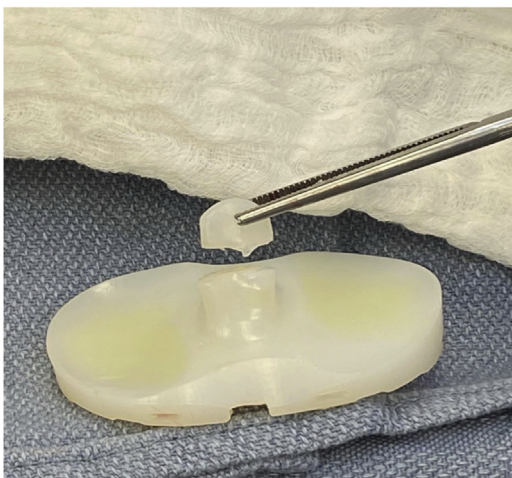
Figure 5. Intraoperative image of an explanted 9-mm Journey 1 BCS tibial polyethylene with a fracture of the tibial post and oxidation of the medial and lateral tibial compartments.
