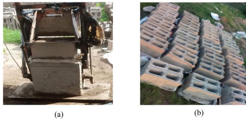
Figure 7. (a) Automated hollow block vibrated compaction (b) Hollow block placement on wooden pallette for curing in natural air and sunlight.
