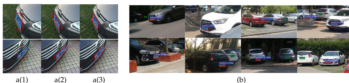
Figure 1. Two main challenges for existing methods. (a) Comparison between different bounding methods (horizontal rectangles, rotated rectangles, and our bounding parallelograms). Existing methods based on horizontal or rotated rectangles cannot tightly enclose the multi-oriented license plates. (b) Representative detection results of Faster R-CNN [27] trained for LPD. The detected regions and actual license plates are presented by red horizontal rectangles and green polygons, respectively. It is difficult to detect license plates with multiple scales, especially the tiny ones.
