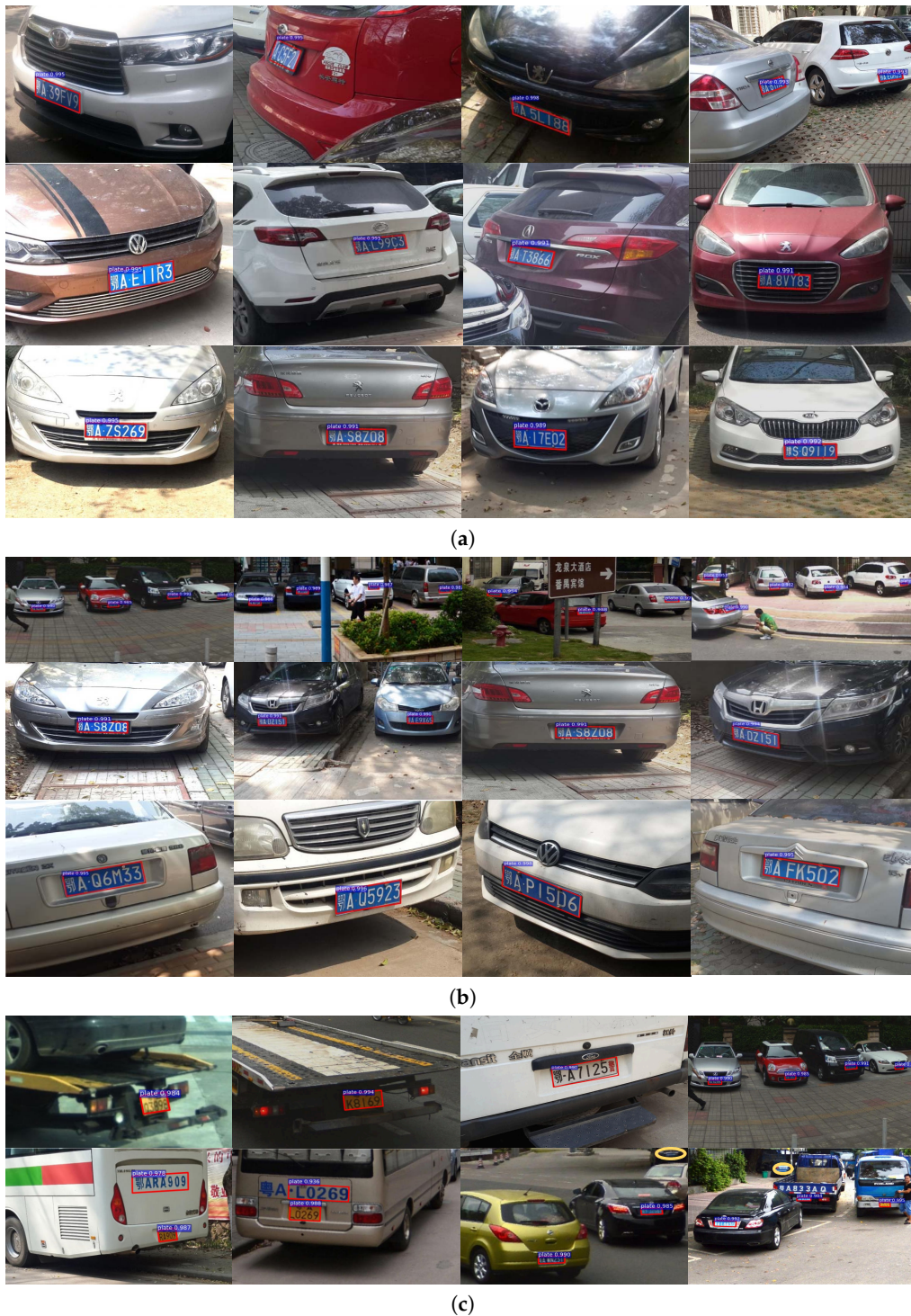
Figure 4. Some representative detection results of our MOSI-LPD: (a) results on license plates with different orientations (skewing violently, modestly and slightly for each row); (b) results on license plates with multiple scales (tiny, medium, and large in scale for each row); (c) results on special or low-resolution license plates in the first row, and scarce cases of mistaking or missing of license plates (indicated by yellow ellipses) in the second row.
