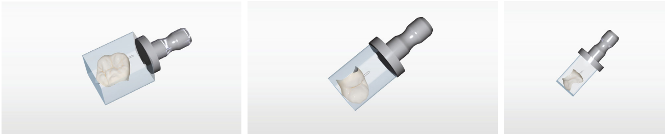
FIGURE 13: Restorations designed for teeth 16, 15, and 14, ready for grinding.
