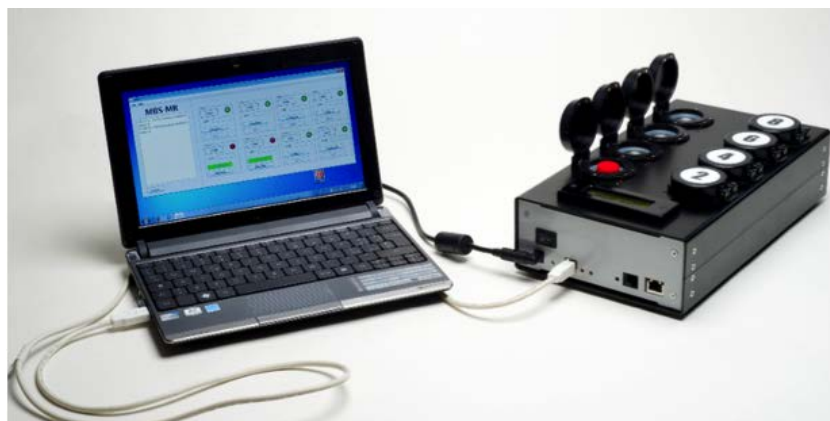
Figure 1. MBS-MR device connected to a computer that is programmed for each day of analysis (Picture from MBS srl).
