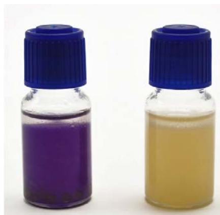
Figure 2. Starting colors blue vial that in the presence of microorganisms changes to yellow color indicating a positive result (Picture from MBS srl).
