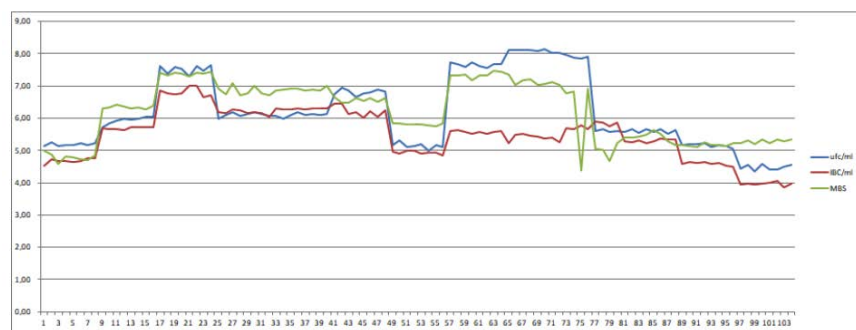
Figure 3. Graphical representation of the trend of the three methods: in blue the plate count at 30°C (CFU/mL), in green the MBS test, in red flow cytometry technology with Bactoscan FC.
