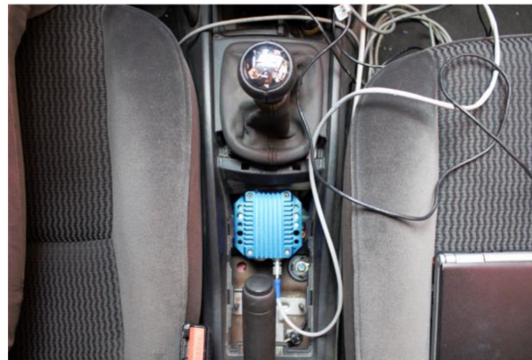
Figure 6. IMU installed inside the vehicle.
