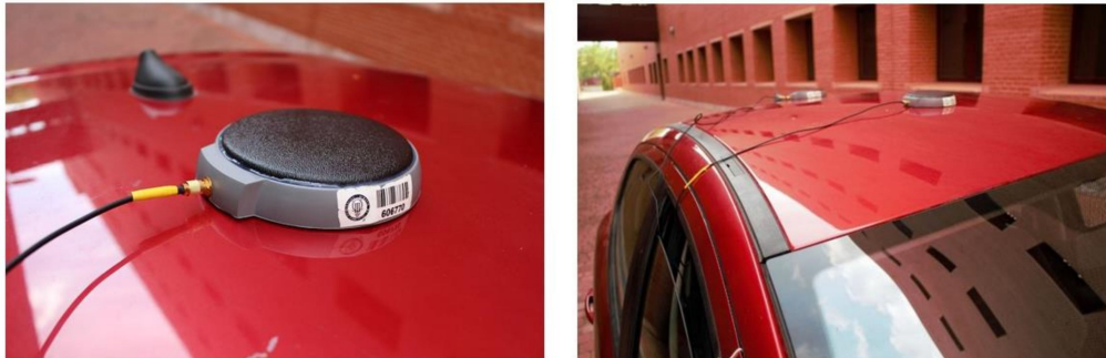
Figure 9. Twin antennas located longitudinally on the roof of the vehicle.
