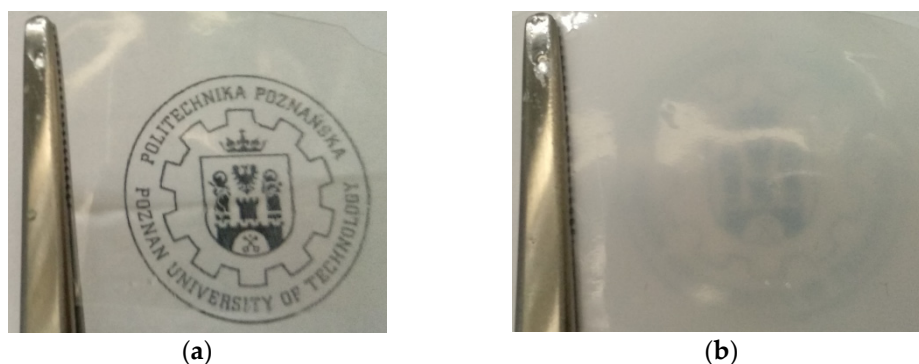
Figure 7. Pictures of materials obtained by the photopolymerization of the composition containing equilibrium mixture of monomers with 50 wt.% of NMP (5Ex:5HP_50) (a) after polymerization, (b) after electrolyte sorption.
