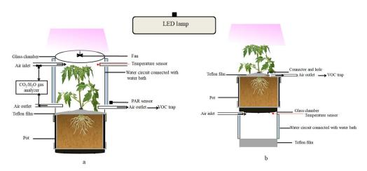
**Figure 4.** Schematic of the dynamic enclosure system used for the measurement of VOC emissions from the entire foliage (**a**) or from the soil surface (**b**) of tomato plants. The arrows indicate the direction of the airflow. The double walled middle section of the chamber with the temperature-regulated water circuit is shown in blue.
