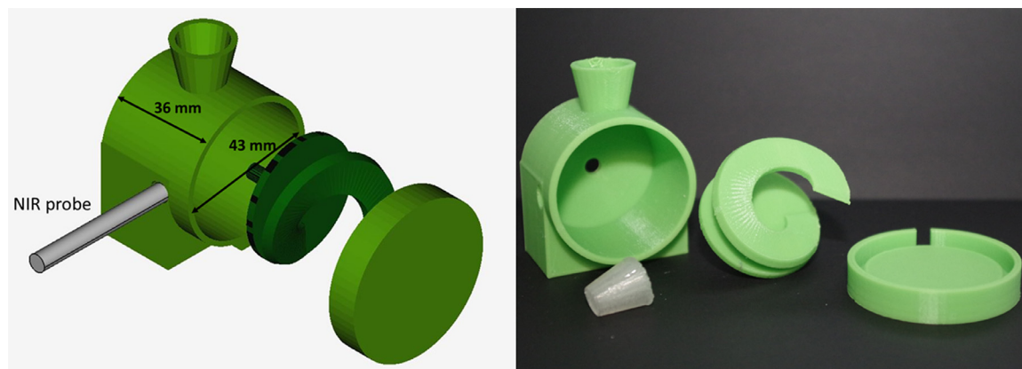
Fig. 1 – Calibration setup left: CAD of the calibration setup, right: 3D printed calibration setup, consisting of chamber, lid, screw and backstopper.
