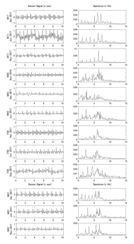
**Figure A2.** The signal waveforms (**left**) measured three times on different days and calculation results of frequency spectrum (**right**) for four people.
