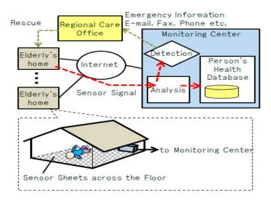
Figure 1. Configuration of elderly home monitoring system.
