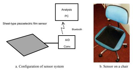
Figure 2. Measurement equipment.
