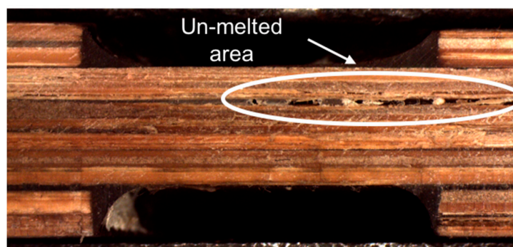
Figure 10. Un-melted area because of the low temperature and time during the melting cycle.
