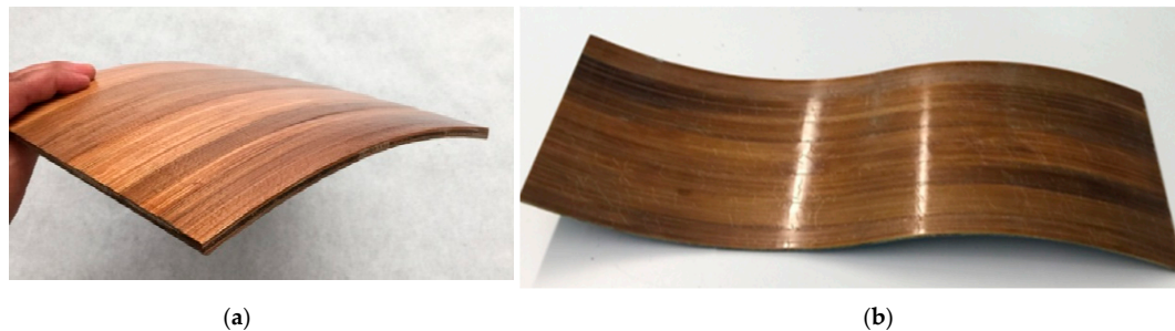
Figure 14. Demonstration panels manufactured from bamboo–PLA composite, (a) Demonstrator 1 cylinder concave shape; (b) Demonstrator 2 concave and convex shape.
