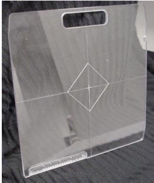
FIG. 1. Diamond template constructed for light and radiation congruence test utilizing an EPID.
