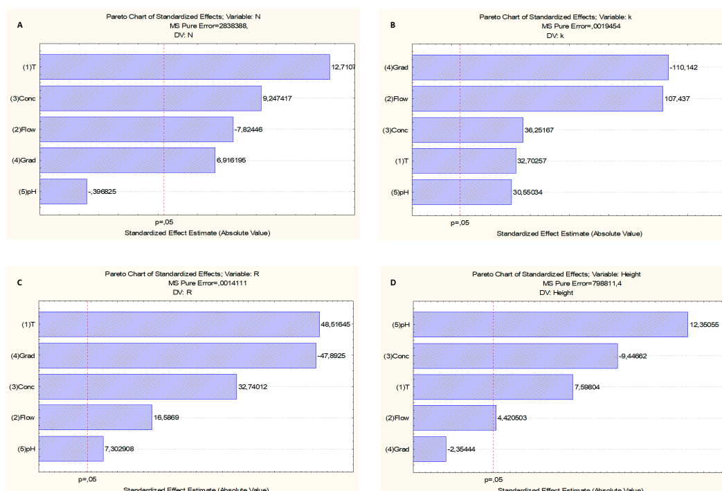
Figure 1. Pareto chart showing the standardized effect of independent variables and their interaction on the (a) Efficiency (N); (b) Retention factor ( k ); (c) Resolution (R); and, (d) Peak height (h). The length of each bar in the chart indicates the standardized effect of that factor on the response. The bar outside the reference line indicates that these terms contribute in the prediction of the dependent variables (N, k , R, and h). The negative coefficients for the model components indicate an unfavorable or antagonistic effect on the variables (N, k , R, and h), while the positive coefficients for the model components show a favorable or synergistic effect on the variables (N, k , R, and h).
