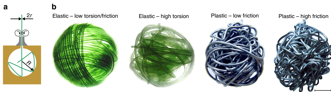
Figure 1 | Experimental set-up and examples of distinct morphologies. (a) Cross-sectional view of the experimental set-up used to compact 1D wires in a spherical rigid container. (b) Distinct morphologies obtained by compacting wires with different material properties introduced in the Methods section. Scale bar, 1 cm.
