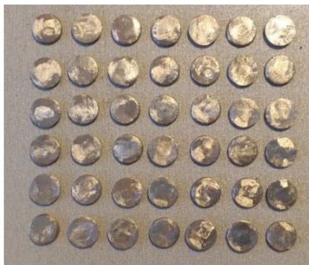
Figure 1. Ni–Cr disc (Suprem Cast V Talladium Inc., Valencia, CA, USA).
