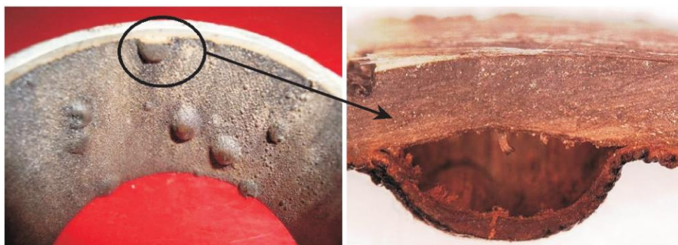
Figure 1. The blister failure of thermoplastic used in oilfield gathering and transportation.
