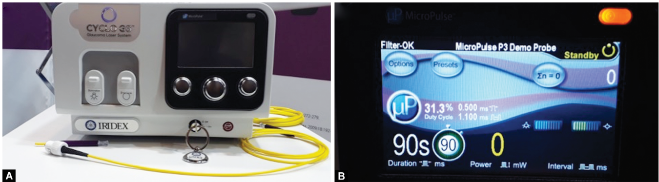
Figs 1A and B: (A) Cyclo G6 Glaucoma Laser System machine (Iridex Corporation, Mountain View, CA, USA); (B) Welcome screen of the machine with a standard 31.3% duty cycle and 90 seconds treatment duration
