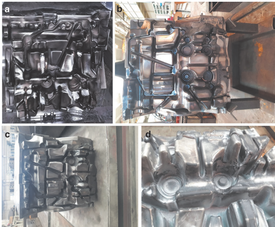
FIG. 21. Soldering of aluminum to the slider (a) serial cooling after 5000 castings. Soldering of aluminum to the slider (b) conformal cooling after 5000 castings. Soldering of aluminum to the slider (c) serial cooling after 40,000 castings. Soldering of aluminum to the slider (d) conformal cooling after 40,000 castings.
