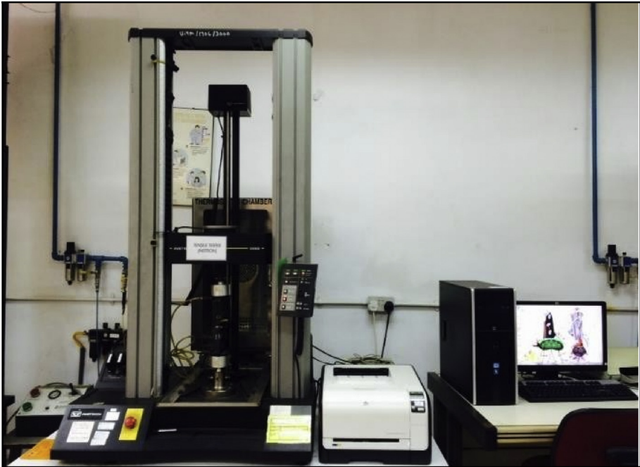
Fig. 5. Set up the tensile instron machine.
